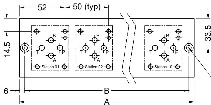
Material : Carbon Steel (Max. Working pressure - 315 bar)
